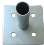
BASE PLATE M36×1.5/150×150×5mm 1.01kg
